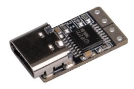
With this small module, you can trigger USB-PD protocols and thus, for example, charge your laptop via a PD-capable USB-C power supply. The output voltage can be adjusted in three steps (5 V, 15 V and 20 V) by setting a resistor.
