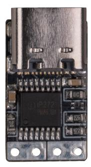
Both resistors soldered = 5 V
