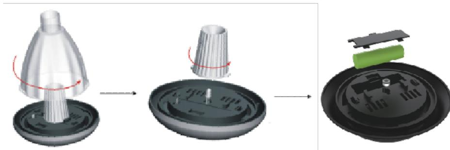
1. Twist and remove the housing ( I ) from the top cover ( II ).
