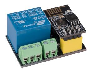
You can freely program this relay module with the help of the attached ESP-01S module and control it remotely via WiFi. This way, for example, smarthome applications such as a light switches can be realised.
