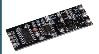
This UART TTL to RS485 converter, allows you to add an RS485 interface to your single board computer. The pin header is included and is not soldered on.
