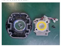
**Step 5**Remove 3x screws and disconnect the PCB
