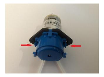
To open the pump module, gently press on the other two clips and remove the pump cover.
