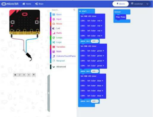
5. Upload the code to your micro:bit. The LEDs should start flashing red, green and blue once the upload has successfully completed, after which you can use capacitive touch keys marked with notes to play a tune!
