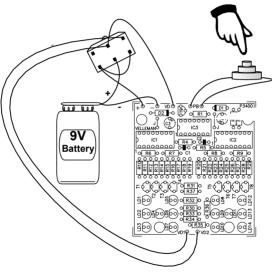
USE A SLIDE SWITCH (ON OFF ON)
