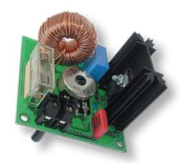
Due to its small size, this small dimmer easily replaces an existing switch, permitting you to vary the brightness of a light or group of lights. The dimmer may also be used to adjust the speed of a motor, vacuum cleaner, or any other motor with carbon brushes. A mains suppresser is provided eliminating undesirable RFI. It is not suitable for halogen lamps.
