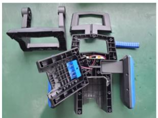
Step 6 Separate the LED casing.
