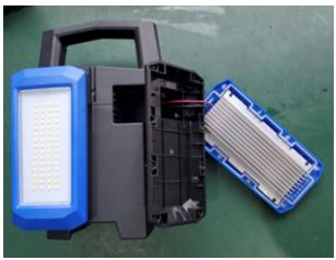
Step 7 Remove the heat sink to access the SMD board.
