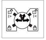
As shown in the figure above, they are wrong settings. In that cases, LED-Un and LED-R will flash at the same time, which indicate the setting error. Normal operation will be resumed through resetting after power -off.
