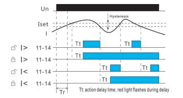
Tr:Power up delay. Tt:Tripping delay.
