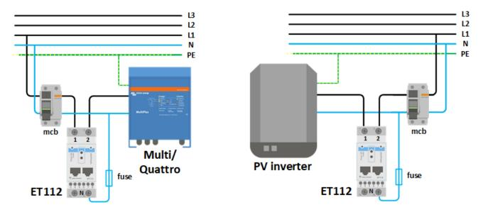
**Grid Meter** - Wiring when used as a grid meter. **PV Inverter** - Wiring when used to measure PV inverter or AC Genset.
