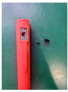
Step 4 Carefully remove the lens.
