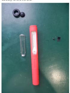
Step 5 Remove the battery, LED and PCB as shown.
