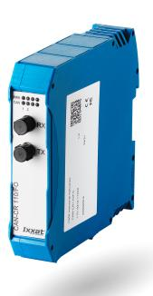
The CAN-CR110/FO repeater with two CAN/CAN FD channels (thereof one as Fiber Optic interface) and integrated bus termination resistors is used for the conversion of the CAN signal from copper wire (ISO 11898-2) to fiber optic cables. It can be used to improve the load capacity of the CAN bus with nodes, to establish a physical coupling of CAN FD bus systems or to insert a galvanic isolation.
