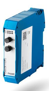
The CAN-CR110/FO repeater with two CAN/CAN FD channels (thereof one as Fiber Optic interface) is used for the conversion of the CAN signal from copper wire (ISO 11898-2) to fiber optic cables. It can be used to improve the load capacity of the CAN bus with nodes, to establish a physical coupling of CAN FD bus systems or to insert a galvanic isolation.
