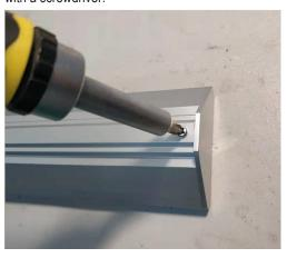
**Step 2**Removes the side plastic cover with a suitable screwdriver.
