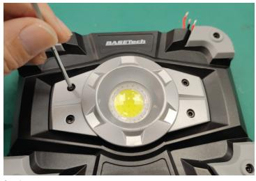
Step 6 Take out the COB and PCB board.
