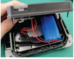
Step 3 Desolder the cables from the battery.
