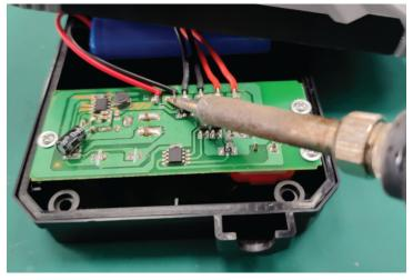
Step 4 Desolder the cables from the PCB board.
