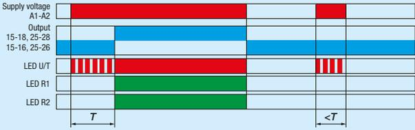
**Ba (OFF-delay with control signal) –** Timing begins when the supply voltage is applied. When the selected time delay (T) is completed the output relay is de-energized. If the supply voltage is interrupted, the output relay is de-energized in case it is energized (after the time delay). If the relay supply voltage is interrupted before the time is completed, the time delay is reset and the output relay won't be energized. This function requires the continuous application of supply voltage.
