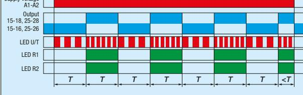
**E (Impulse ON) –** The output relay is immediately energized when the supply voltage is applied and de-energized when the selected time (T) is completed. If the supply voltage is interrupted before the time delay is completed, the relay is de-energized and the time delay is reset. This function requires the continuous application of supply voltage.
