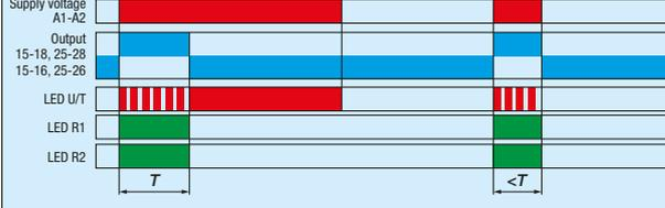
**Fa (Impulse ON with control signal) –** The output relay is energized after the control supply voltage is applied and de-energized when the time delay (T) is completed. If the supply voltage is interrupted before the time delay is completed, the relay is de-energized and the time delay is reset. This function requires the continuous application of supply voltage.
