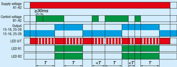
**Da (symmetric flasher, start ON) –** Applying the supply voltage, timing begins with times given by T1 (output ON) and T2 (output OFF). The cycle starts with the output relay energized. The times of full scale range T1 and T2 are the same. The total cycle is given by  $T = T1 + T2$ . Interrupting the supply voltage with the output energized resets the time delay and de-energizes the output relay. This function requires the continuous application of supply voltage.
