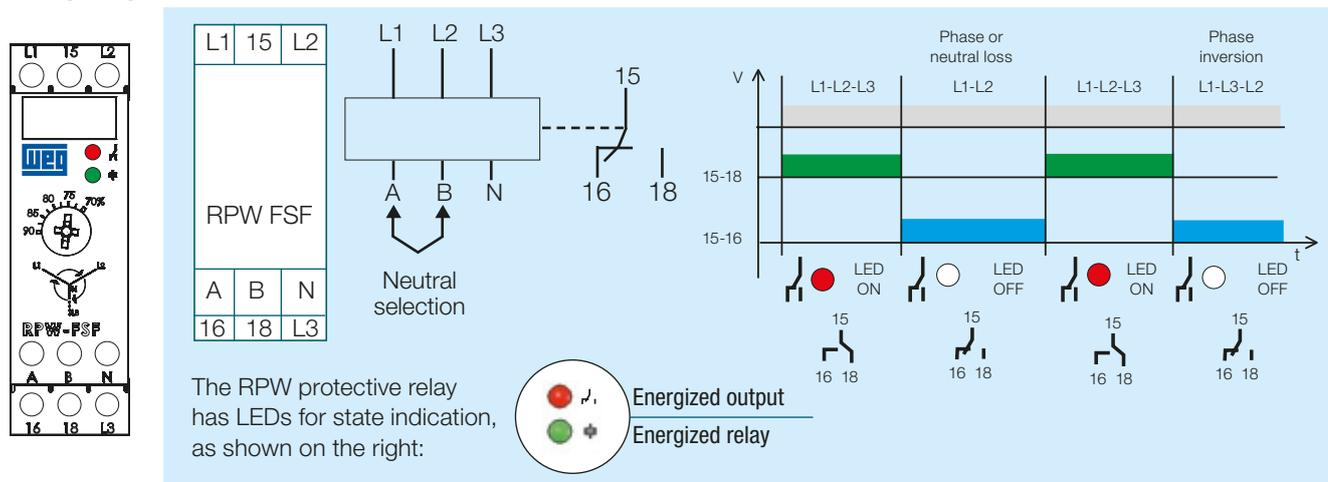
Note: for application in generator sets, frequency inverters with 12-pulse or regenerative rectifiers, electronic power controllers (dimmers or the like) or where a high level of harmonic currents may be present (above the recommendation of IEEE519), we recommend the ERWM relay.
