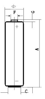
Capacity: 3000 mAh (10 mA, 24 h/d, 20°C, e.v.= 0.8 V)
