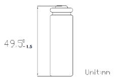
Capacity: 1400mAh (Charge 140 mAx16h ;Discharge 280mA to 1.0 V;at 20°C)
