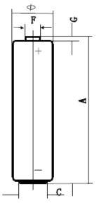
Capacity: 1350 mAh (10 mA, 24 h/d, 20°C, end voltage = 0.8 V)
