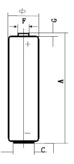
Capacity: 2500 mWh (15 mA, 24 h/d, 20°C, e.v.= 1.0 V)
