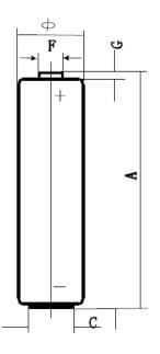
Capacity: 2750 mAh (27.5 mA, 24 h/d, 20°C, e.v.= 1.0 V)
