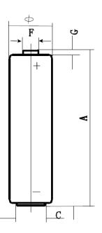
Capacity: 50mAh (10k Ω,24h/d, 20°C, e.v.:6.0V)
