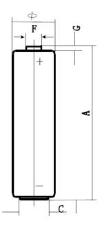
Capacity: 20 mAh (20k Ω,24h/d, 20°C, e.v.:6.0V)
