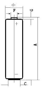
Capacity: 500mAh (35mA, 24h/d, 20°C, e.v.= 0.8V)
