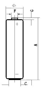
Capacity: 3000 mAh (10 mA, 24 h/d, 20°C, end voltage = 0.8 V)
