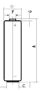
Capacity: 1100 mAh (30 mA, 24h/d, 23°C±2°C, e.v.= 0.9V)
