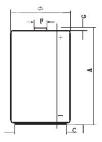
Capacity: 7500 mAh (25 mA, 24 h/d, 20°C, end voltage = 0.8 V)
