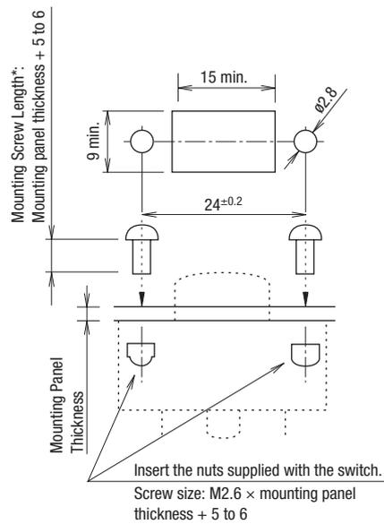
Note: When installed on a mounting panel thicker than 2 mm, the actuator surface is below the panel when the button is pressed to position 3.
