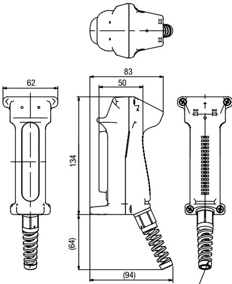
Cable Gland (supplied with grip style enabling switch)
