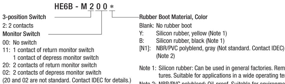
Note 1: Silicon rubber: Can be used in general factories. Remaining flexible in cold temperatures. Suitable for applications in a wide operating temperature range.
