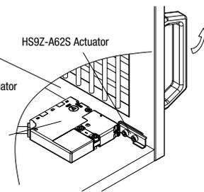
Note: When mounting an actuator, make sure that the actuator enters the slot in the correct direction, as shown on the right.
