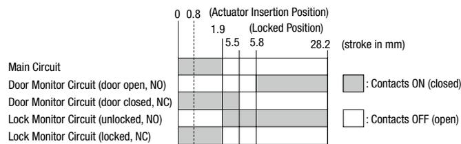
• The characteristics shown in the chart above are of the HS9Z-A61, -A62, -A65, and -A66 actuators.
