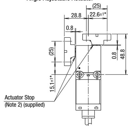
Note 2: Remove the actuator stop after mounting the actuator.
