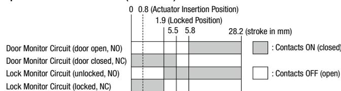
• The characteristics shown in the chart above are of the HS9Z-A61, -A62, -A65, and -A66 actuators. For the HS9Z-A62S actuator, subtract 0.6 mm.
