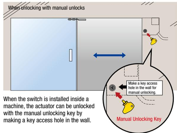
When the switch is installed inside a machine, the actuator can be unlocked with the manual unlocking key by making a key access hole in the wall.
