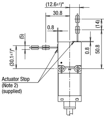
Using the HS9Z-A62 Right-angle Actuator
