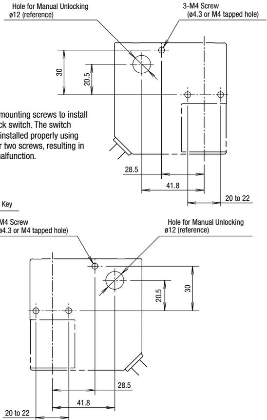
Use three mounting screws to install the interlock switch. The switch cannot be installed properly using only one or two screws, resulting in possible malfunction.
