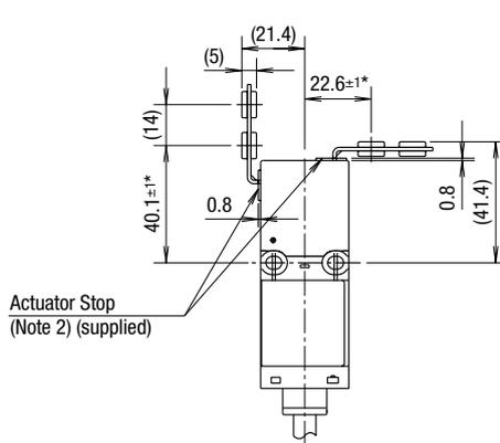
Using the HS9Z-A65/A66 Angle Adjustable Actuator
