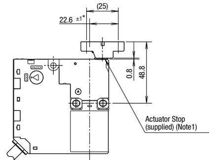
Note 1: Remove the actuator stop after mounting the actuator.
