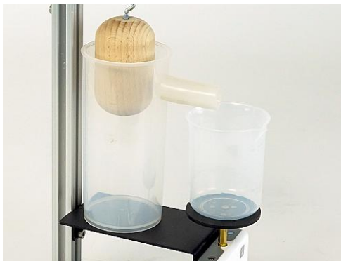
Fig. 10 Container with drain
