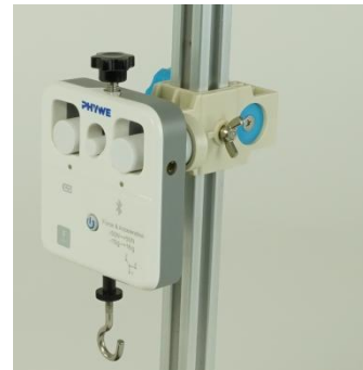
Fig. 14 Height adjuster with wing screw
