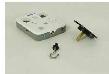
Fig. 7 Sensor with hook and weight plate
