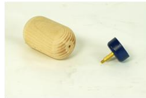
Fig. 11+12 Float and sensor with magnet
