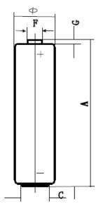
Capacity: 1350 mAh (10 mA, 24 h/d, 20°C, end voltage = 0.8 V)
