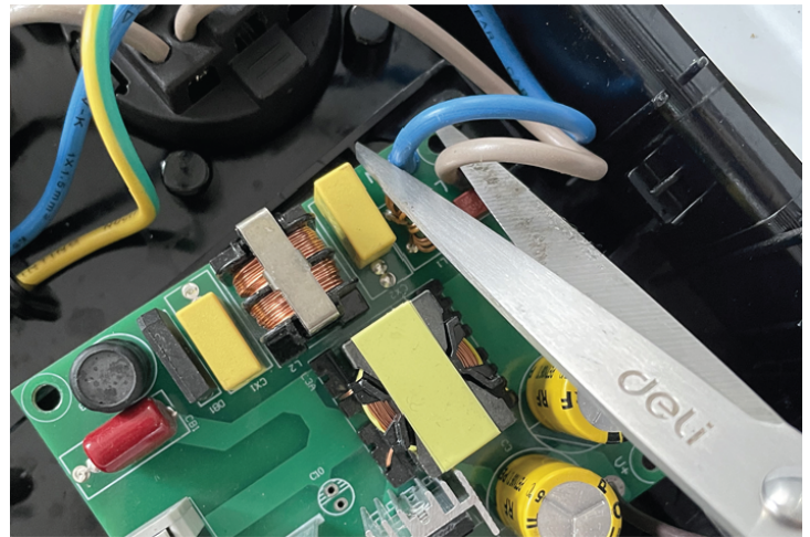
Step 12 Remove the driver with LED module for SLR testing.
