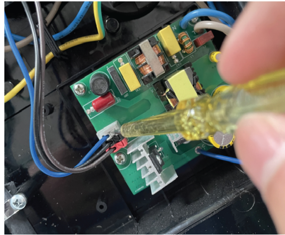
Step 9 Short-circuit the grey and black connection terminals with the wire.
