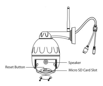
The record files of the IP camera can be stored in the Micro SD Card.
