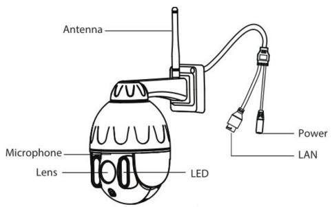
LED: 6pcs Infrared-LEDs, night vision range up to 50 metres / 164ft.
