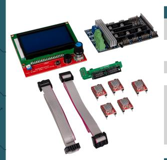
With this complete set, you lay the foundation for installing your own Arduinobased 3D printer.
