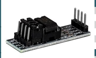
This EEPORM memory allows you to store and read data externally via the I2C interface of your microcontroller.
