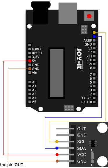
The analog output of the converter is at the pin **OUT**.
