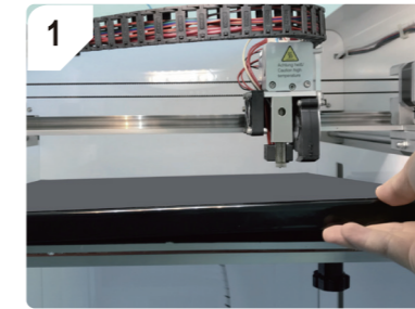
Insert the print bed and magnetic mat.
