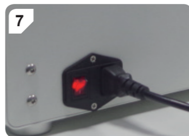
1. Connect the mains cable to the power inlet on the printer. 2. Flip the power switch into the position I to switch on. The display lights up.
