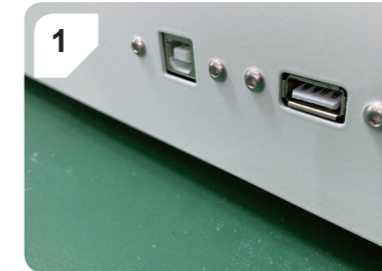
Connect the USB memory stick that contains the print file to the USB port.
