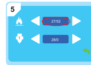
Wait until the preheat temperature has been reached.
