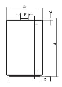
Capacity: 18000 mAh (25 mA, 24 h/d, 20°C, end voltage = 0.8 V)
