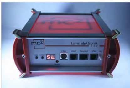
Track voltage = off
