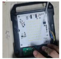
Unscrew 4x light source board screws.
