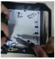
Unsolder the connection between the power cord and light board.
