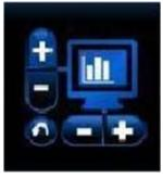
and – control the time scale. Clicking the reverse arrow icon (bottom-left) clears the screen and allows a fresh plot of data to be displayed.
