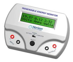
There are two sets of **Input** and **Output** terminals. The **Input** terminals are on the left side and the **Output** terminals are on the right side of the unit. The Red terminal is + or positive while the Black terminal is – or negative. You must observe the correct polarity when hooking up batteries, solar panels, wind turbines or fuel cells to the terminals.
