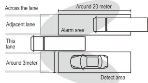
2.2.1 When normal driving, if there is another vehicle closing to the left (right) side of the vehicle, the left(right) LED light will flash. No buzzer alarm.
