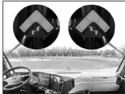
5.8.2 The buzzer affixed inside plastic of the main driving, make sure a sound output
