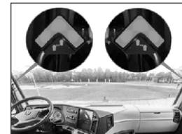
6.2.2 After the system enters the working condition, to detect both sides of the car rear side blind area (covering both sides of lane, the length about 20 meters).
