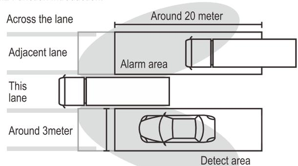
2.2.1 When normal driving, if there is another vehicle closing to the left (right) side of the vehicle, the left(right) LED light will flash. No buzzer alarm.
