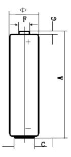
Capacity: 1350 mAh (10 mA, 24 h/d, 20°C, end voltage = 0.8 V)
