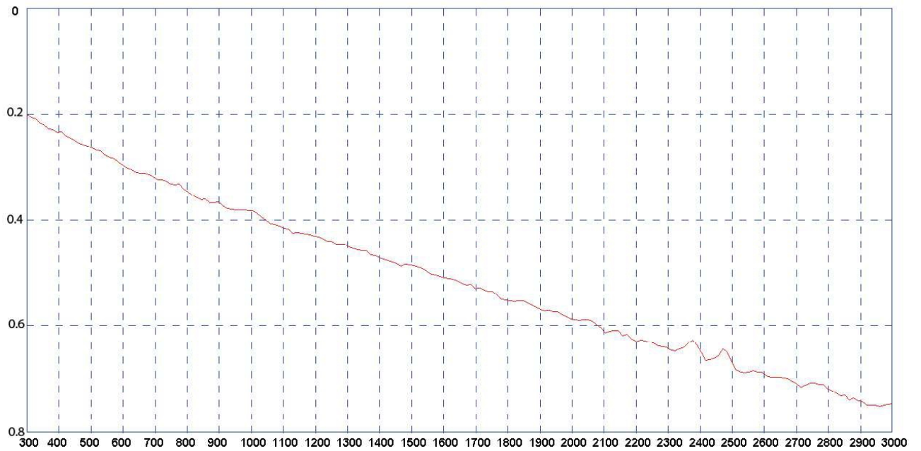
Typical Attenuation dB per m of Cable*
