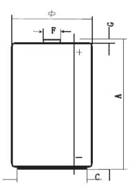
Capacity: 8000 mAh (25 mA, 24 h/d, 20°C, end voltage = 0.8 V)
