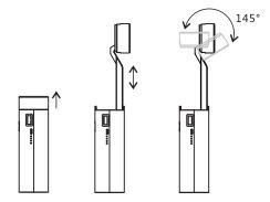
The lamp shade can be adjusted many angles, and the telescopic neck can extend the lamp head up and down.
